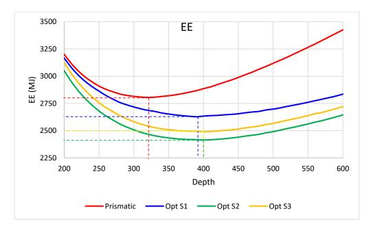
For Prismatic vs Optimised beams, Optimum depth changes!!
