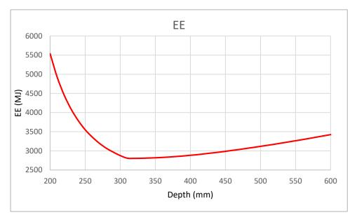
With this kind of graphs, the optimum depth for a given set of conditions can be identified, hence the minimum embodied energy possible for the selected construction technique.
